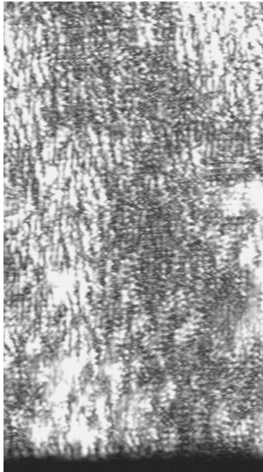
C Scan Image Pitch – catch at 0.25 mm pitch
