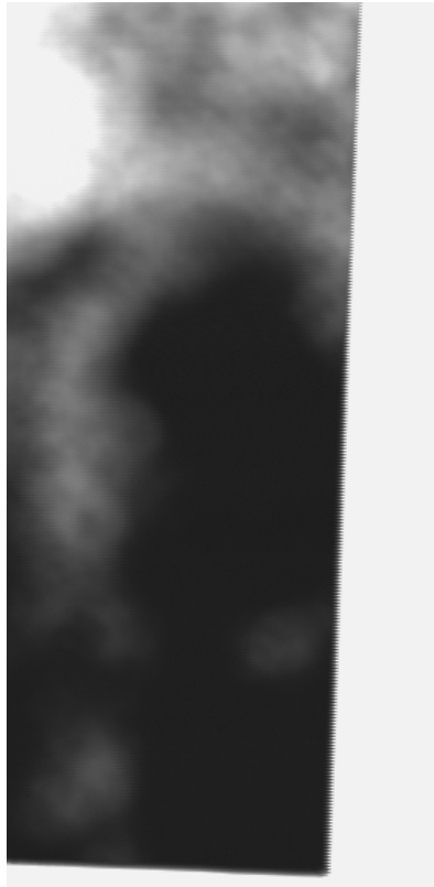
C Scan Image Through Transmission at 0.25 mm pitch, 18 dB Gain
